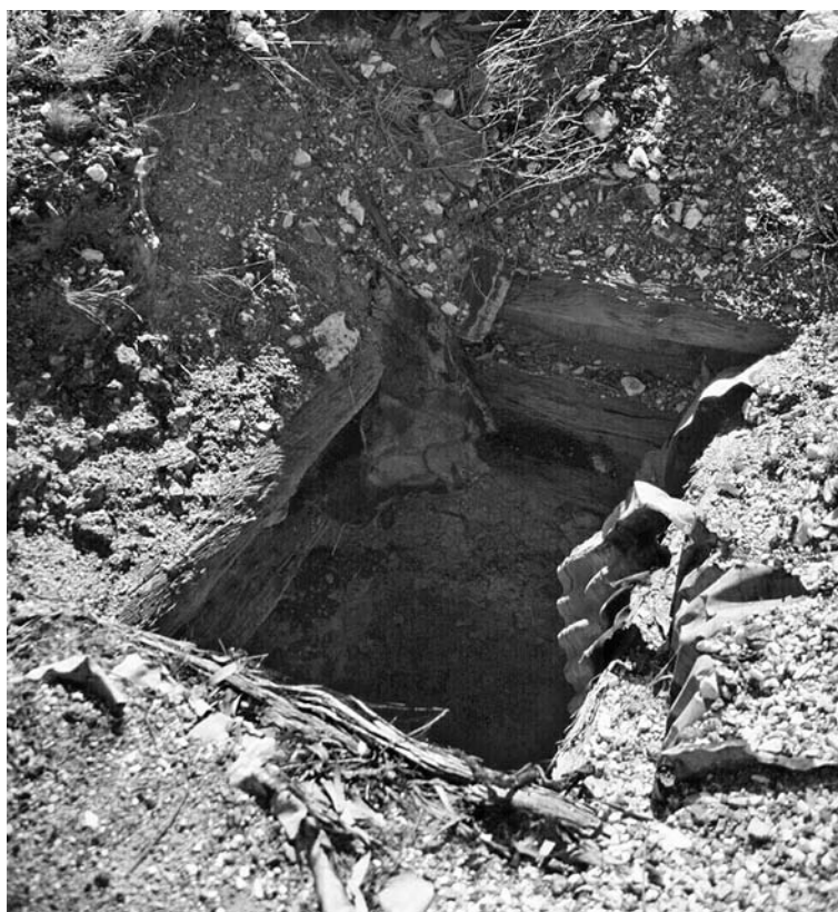
Fig. 35: Unsecured, open shaft in the abandoned Coolgardie/Australia gold mining field.
