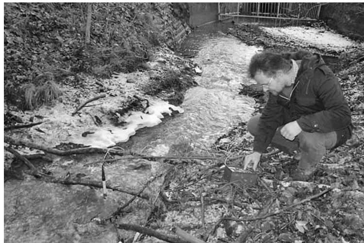
Fig. 61: Flow measurement with the salt dilution method in the turbulent flowing German Gernrode/Harz Steinbach creek. The salinity probe is hanging in the middle of the stream and the data logger records the electrical conductivity every second (photograph Andrea Berger).
