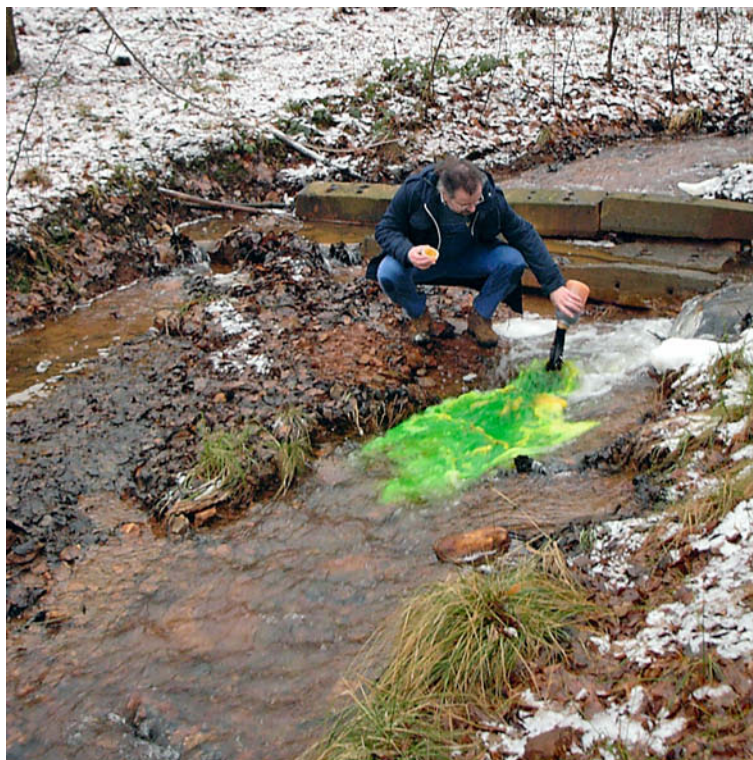
Fig. 48: Flow measurement with Na-fluorescein at the inlet of a lake which receives polluted mine water. Shown is the Dirac-impulse injection of the Na-fluorescein (dark colour when it flows out of the bottle, lighter colour when it mixes with the stream water; photograph Andrea Berger).
