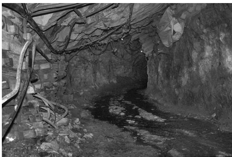
Fig. 18: Unflooded access Gallery in the Western Deep Level/South Africa underground mine. The Gold Reef comes in from the top right side and dips to the lower left corner. Concrete support helps to support the geomechanical stability in the 2500 m deep gallery.
