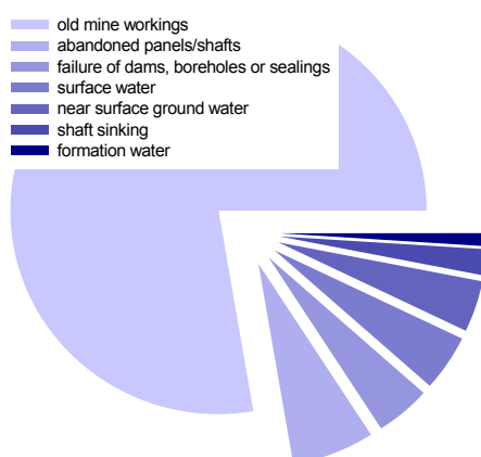
Fig. 19: Reasons for mine inundation (modified after Job 1987; Vutukuri and Singh 1995).
