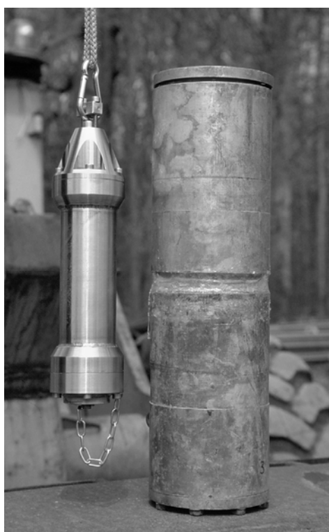
Fig. 63: Tracer Injection Apparatus (TinA, left) and Lycopodium Apparatus (LydiA, right). The Diameter of LydiA is 120 mm.
