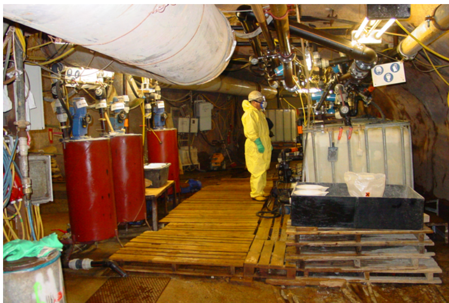
Fig. 5. Immobilization grout plant 2005, capacity up to 50 \text{ m}^3/\text{h} , solution vessels on the left site, mixing facilities on the right site, storage vessels in the background.
