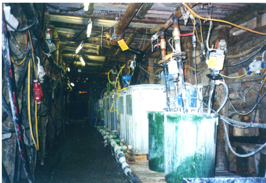
Fig. 4. View of the grout plant used for field tests and first full scale application.
