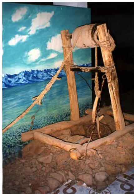
Photograph 1. A windlass is used to bring tunnel spoil to the surface (display at the Qanat Museum in Turpan, China).
